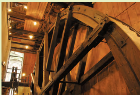
Kamšt – the massive wooden water wheel with a diameter of 13.6 metres, one of the most significant technical monuments in Slovenia and the largest preserved device of its type in the world.
